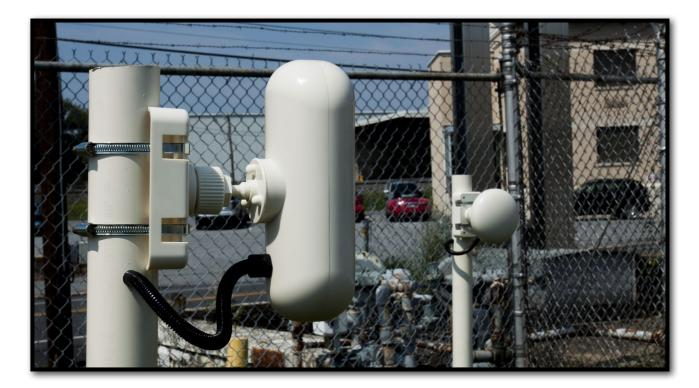
The **Predix™** detector is a linear barrier based on K-band microwave technology. It is comprised of a transmitter and receiver, which together establish perimeter protection with coverage up to 300 meters. It is very simple to install, yet provides a high level of security performance. The microwave signal is digitally converted and analyzed by a microprocessor using an innovative and efficient algorithm.
